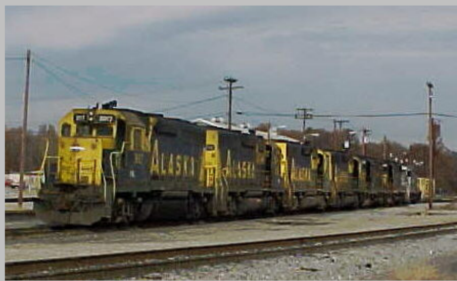
Fodder for P&L's slug program. 4 Alaska RR GP40s and 2 GP35s. The units were spotted at the P&L engine facility in Paducah on November 28, 2000. The GP40s will be slug mothers and the GP35s slugs. Digital image Chuck Hinrichs
